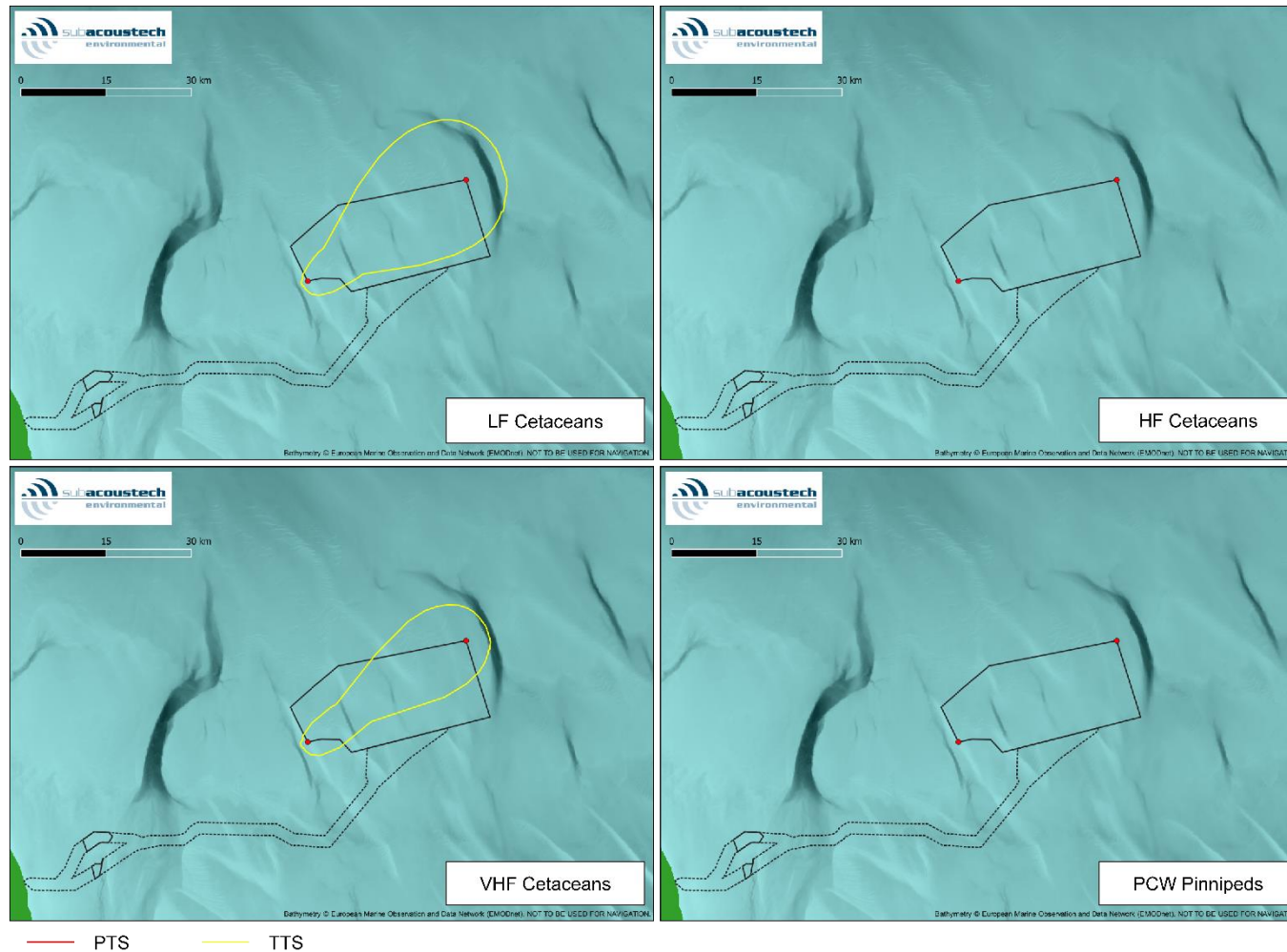
Figure A 1 Contour plots showing the in-combination impacts of simultaneous installation of monopile foundations at the SW and NE modelling locations for marine mammals using the non-impulsive Southall et al. (2019) criteria assuming a fleeing animal
